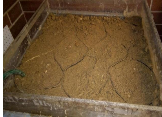
Figure 3.28 Geocell Installation in HGRS Section
