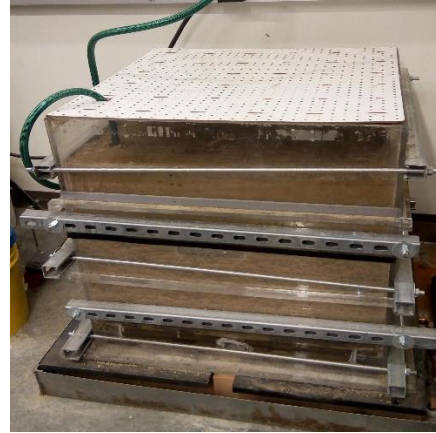
Figure 3.16 Control Section after Compaction
