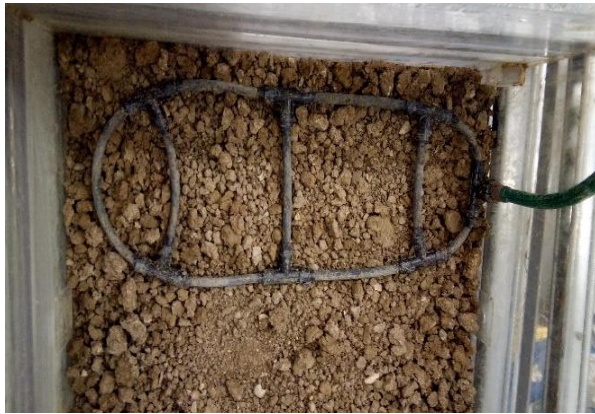
Figure 3.4 Soaker System Arrangement
