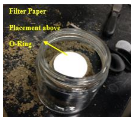
Figure 4.4 Soil Specimen Prepared for Total Suction Measurement
