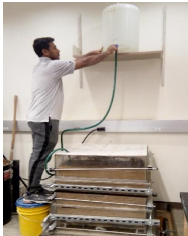
Figure 3.17 Moisture Supply through Water Reservoir
