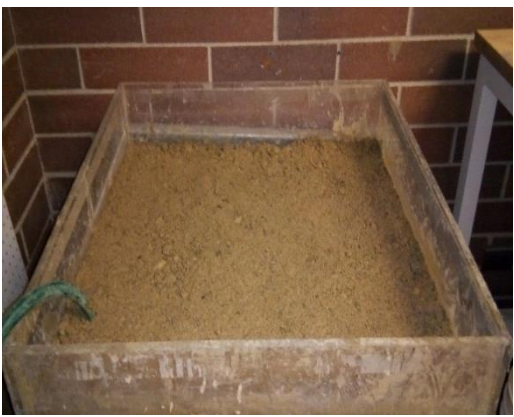
Figure 3.21 GC Section after Compaction
