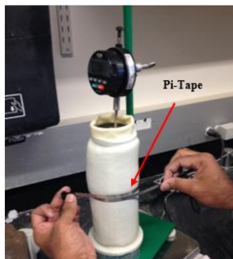
Figure 4.8 Measurement of Radial Swell using Pi-Tape
