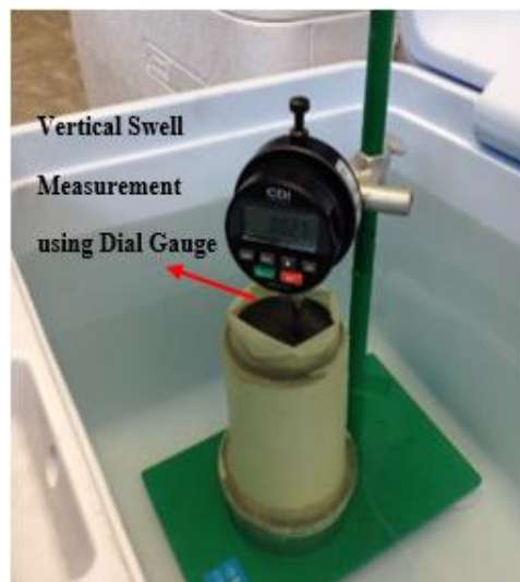
Figure 4.7 Inundation of Soil Sample in Water Bath
